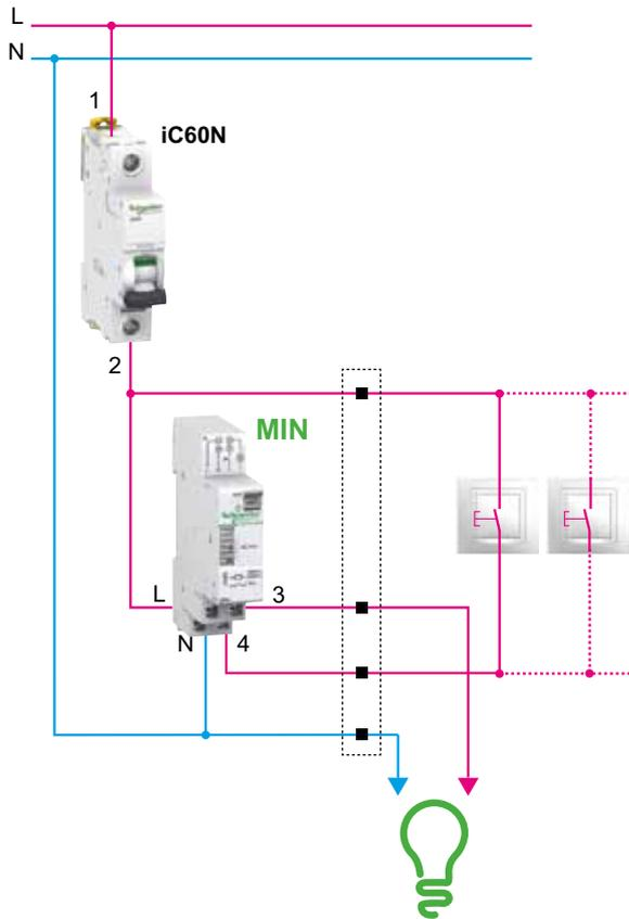
Connection to 3-conductor riser pipe
