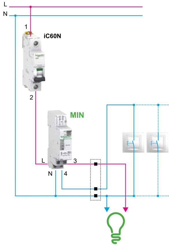
Note: 3 or 4 wire connection to be selected using the lateral selector switch of MIN.
